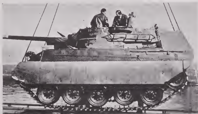
FIGURE 6. Experimental installation of simple track shrouding for submerged track propulsion study on T-70 gun motor carriage.
